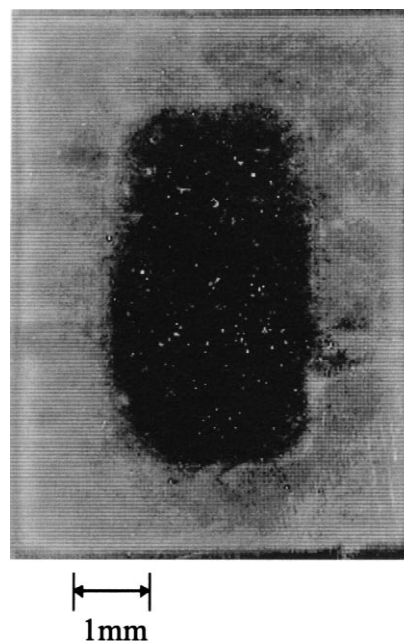
Fig. 3. \alpha -Autoradiograph taken from the polished surface of a sectioned spinel pellet following infiltration of a plutonium nitrate solution for 30 s.
